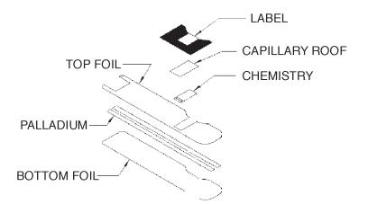
FIG. 2. An exploded view of the Accu-Chek<sup>™</sup> Comfort Curve<sup>™</sup> biosensor test strip.
