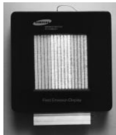
Fig. 4. Carbon nanotube-based 4.5-inch field emission display unit. (Reprinted with permission from Dr. Wong Bong Choi and Samsung Advanced Institute of Technology.)
