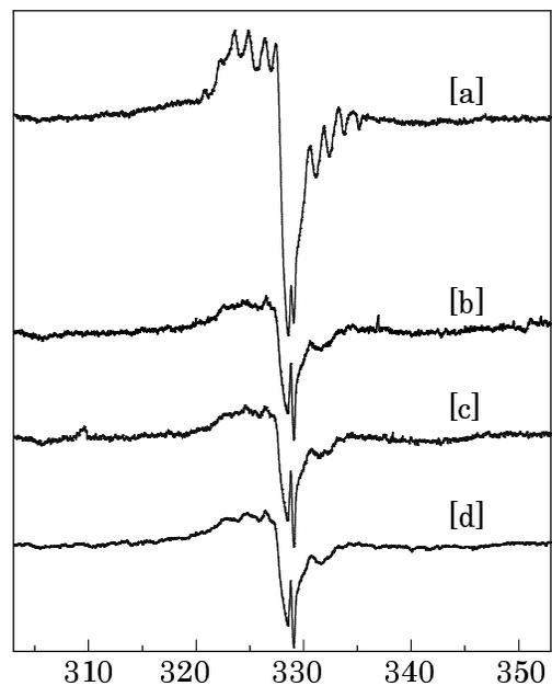
Fig. 2 EPR spectra [a] uv-irradiated [b] 5 min [c] 30min and [d] 3h of Sr<sub>0.995</sub>Dy<sub>0.005</sub>Al<sub>2</sub>O<sub>4</sub> and this decay characteristic at room temperature.
