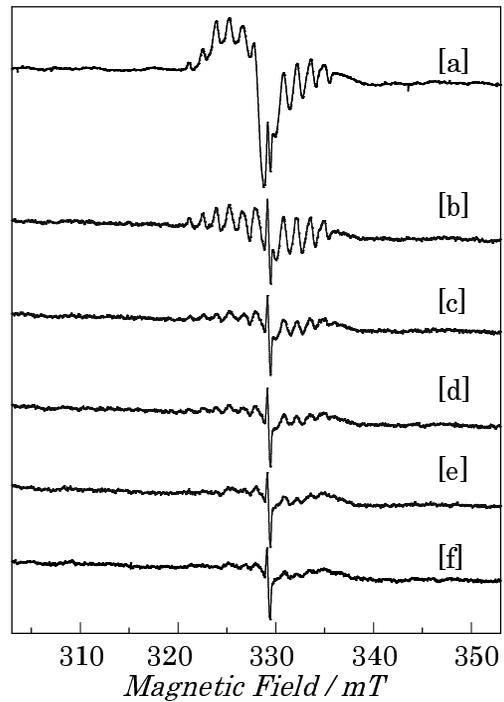
Fig. 1 EPR spectra [a] uv-irradiated [b] 5 min [c] 30min [d] 1h [e] 3h and [f] 6h of SrAl<sub>2</sub>O<sub>4</sub> and this decay characteristic at room temperature.
