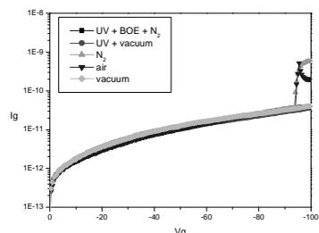
Fig. 3. Ig-Vg characteristic curves for various pre-treatment conditions.
