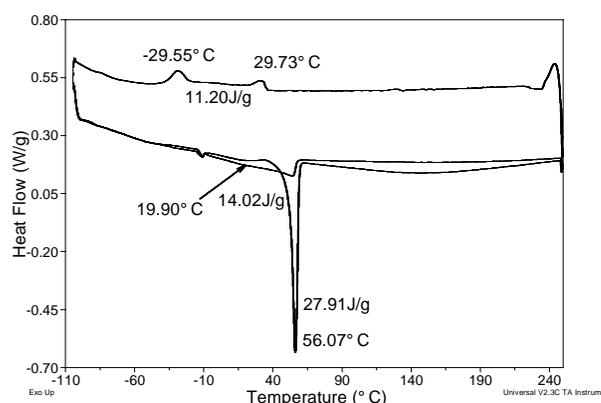
Figure 2. DSC trace of PEO(4600)/R812s(surface methyl groups) fumed silica blend in 30/70 wt ratio
