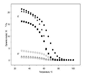
Fig. 1. Temperature dependence of dynamic moduli of gel electrolytes based on PMMA and fumed silica in LiCF<sub>3</sub>SO<sub>3</sub>/PC system. (**■**) Without fumed silica, ( $\blacktriangle$ ) With fumed silica A380 (1.3%), (**●**) With PMMA grafted A380 (1.3%). Upper curves: storage moduli, E'; lower curves: loss moduli, E''. Test frequency: 1 Hz.
