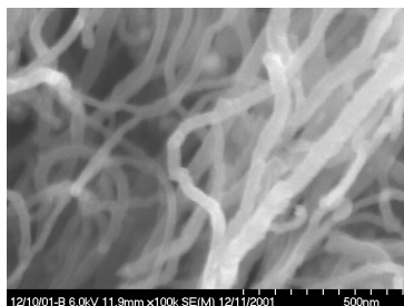
Fig. 1. SEM image of multi-wall carbon nanotubes synthesized by catalytic decomposition of C 2 H 2 .
