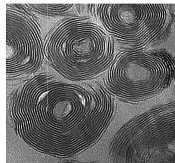
Figure 1. TEM micrograph taken perpendicular to the axis of the nanotubes. The scroll-like structure of the vanadium oxide nanotubes can be clearly seen. The displayed material was synthesised with hexadecylamine ( \text{C}_{16}\text{H}_{33}\text{NH}_2 ) as template.
