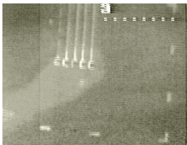
Fig. 2 Fluorescent microscopy image of OH - production in solution at Cu islands on individual Al electrodes.
