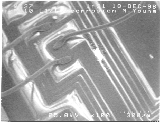
Figure 2. Scanning Electron Micrograph of Aluminum trace corrosion.
