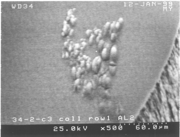
Figure 3. Scanning Electron Micrograph of Aluminum corrosion on ZnO transducer electrode.
