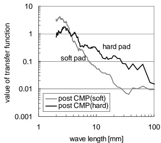
Fig.3 Calculated transfer functions as the ratio of PSD of the oxide film thickness variation to that of nanotopography using soft pad and hard pad. The removal depth was set to 3000Å.
