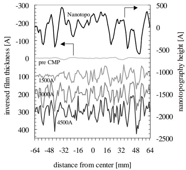
Fig.1 Nanotopography and film thickness profiles before/after CMP through the reiterated polishing of one wafer using a soft pad.
