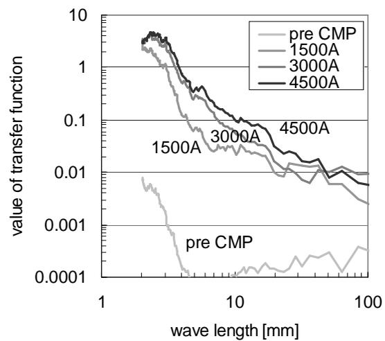
Fig.2 Calculated transfer functions as the ratio of PSD of the oxide film thickness variation to that of nanotopography using soft pad. The removal depth dependency is shown in the figure.
