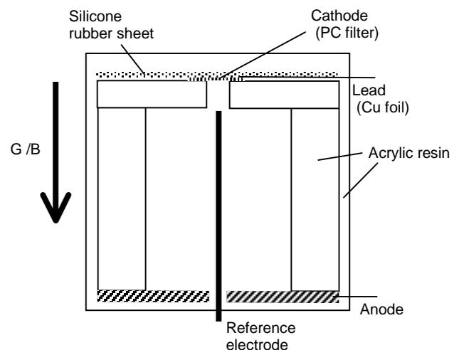
Fig.1: Schematic illustration of electrolytic cell (C/A configuration).
