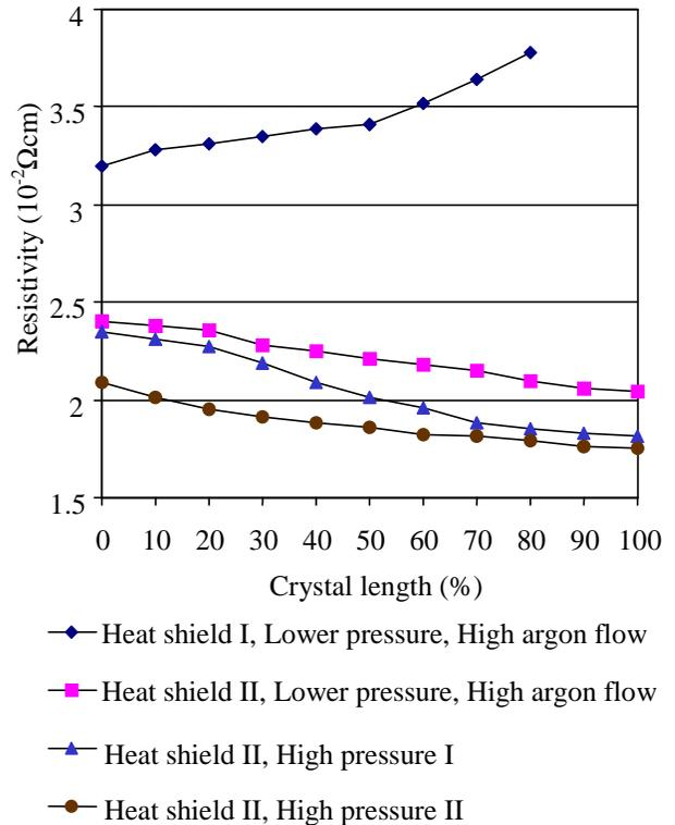
Figure 1 Resistivity profiles along with the crystal growth direction
