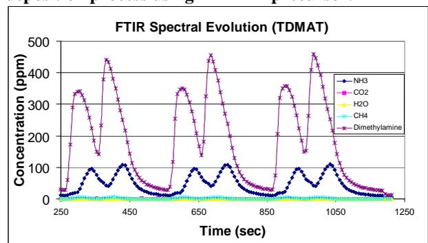
**Figure 3: Spectra from the inlet and outlet of abatement device on TDMAT process.**
