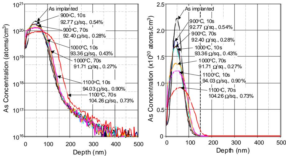
Fig. 1. SIMS depth profiles of <sup>75</sup>As<sup>+</sup> implanted wafers after annealing using a lamp-based RTA system. (<sup>75</sup>As<sup>+</sup> 70keV, 1x10<sup>15</sup>atoms/cm<sup>2</sup>)
