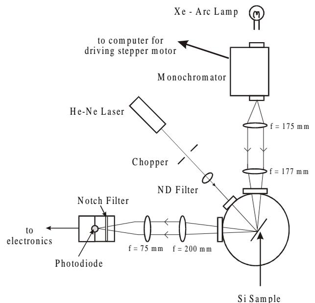
Fig. 1 – Schematic of photoreflectance setup.
