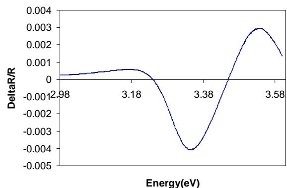
Fig. 2 – Sample PR spectrum taken in our laboratory from n-doped Si.
