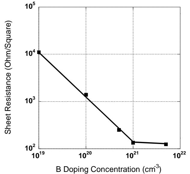
Fig. 1. Sheet Resistance of as-grown 10 nm B-doped Si
