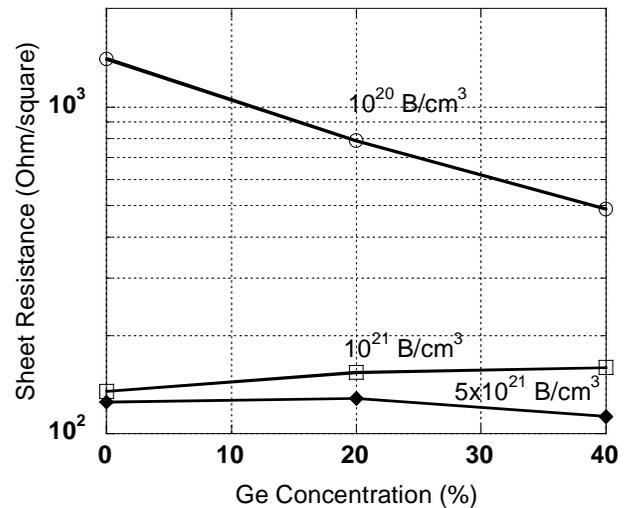
Fig. 2. Effect of Ge Concentration on the sheet resistance of 10 nm layers of  $\text{Si}_{1-x}\text{Ge}_x$  ( $x = 0, 0.2,$  and  $0.4$ ).
