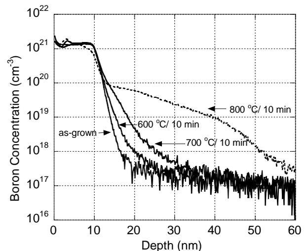
Fig. 3. Thermal stability of B-doped  $\text{Si}_{0.6}\text{Ge}_{0.4}$  after a 10 minute furnace anneal.
