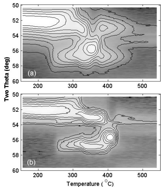
Fig.2 *In situ* x-ray measurement during annealing of a 10 nm Ni film deposited on (a) n-doped and (b) p-doped SOI substrate.
