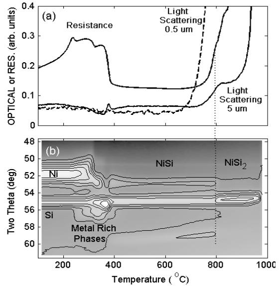
Fig. 1 (a) Resistance and light scattering from 0.5 and 5 μm length scales together with (b) x-ray diffraction measurements performed *in situ* during annealing (3 °C/s) of a 10 nm Ni film deposited on n-doped poly-Si.
