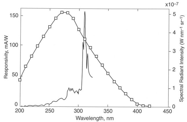
Figure 1: SiC Photodiode UV responsivity and UV flame emission spectrum
