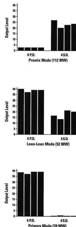
Figure 3: Primary and Secondary Zone Flame Sensor Output Signal Levels for Dry Low NOx Oil Burning Gas Turbine During Power Plant Operation
