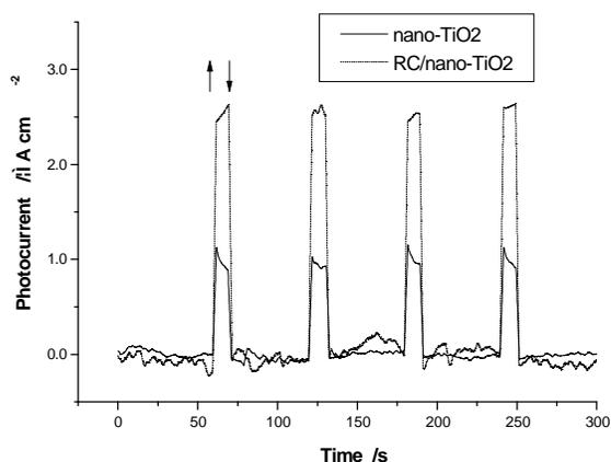
Figure 2 Short-circuit photocurrent changes induced by switching on (↑) and off (↓) the illumination for the RC/nano-TiO<sub>2</sub> and nano-TiO<sub>2</sub> film.
