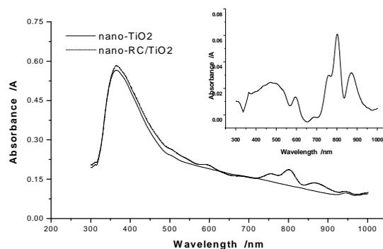
Figure 1 Absorbance spectra for nano-TiO<sub>2</sub> and RC/nano-TiO<sub>2</sub> film. The insert showed the difference spectrum of the two films.
