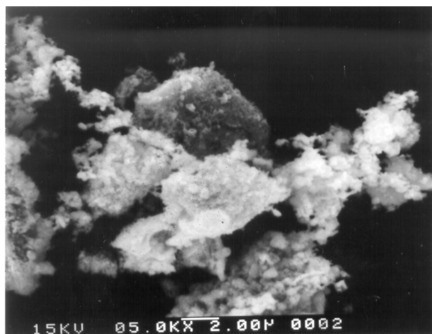
Figure 1. Scanning electron micrograph of a \text{LiAl}_{0.25}\text{Mn}_{1.75}\text{O}_4 spinel made by a sol-gel method using \text{Li}_2\text{S} .
