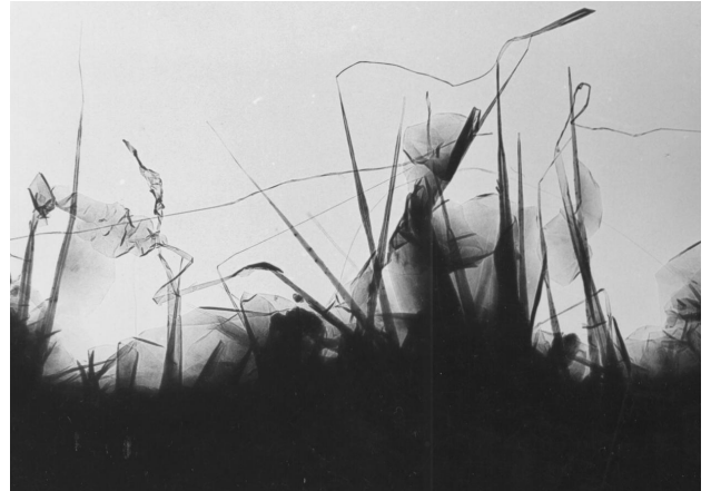
Fig.1. TEM image of carbon film produced in DC discharge in methane-hydrogen atmosphere.
