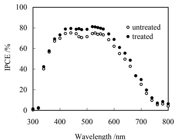
Fig. 1 Photocurrent action spectra of  $\text{RuL}_2(\text{SCN})_2$  sensitized electrodes with and without the post-treatment
