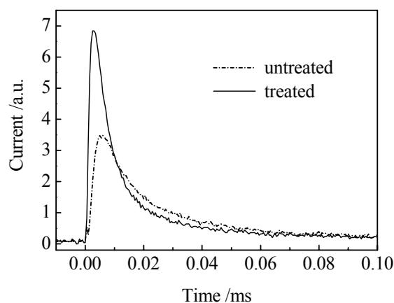
Fig. 2 Photocurrent transients of  $\text{RuL}_2(\text{SCN})_2$  sensitized electrodes with and without the post-treatment
