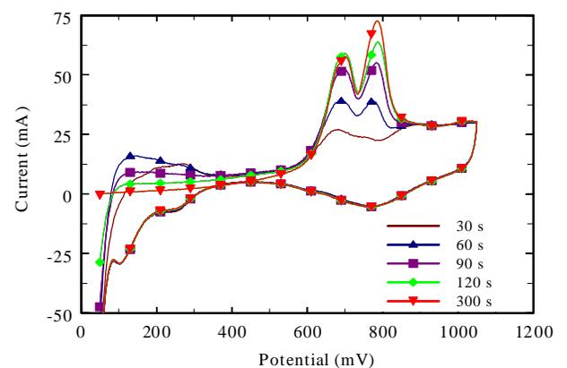
**Figure 1:** Cyclic voltammetry on a Pt composite electrode at room temperature under atmospheric N<sub>2</sub> flow after various exposure times to CO. The total flow rate was 0.1 SLM. The symbols correspond to time duration indicated by the legend.
