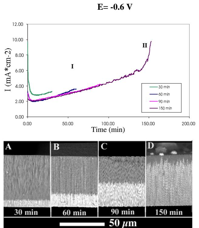
**Figure 1.** Bottom: SEM images (back-scattered electrons) showing cross-section of Cu-filled membranes following regular Cu electrodeposition for several time periods (indicated). Top: Reduction current density as a function of time of deposition. Electrodeposition was carried out at  $-0.6$  V vs. Hg/Hg<sub>2</sub>SO<sub>4</sub>.
