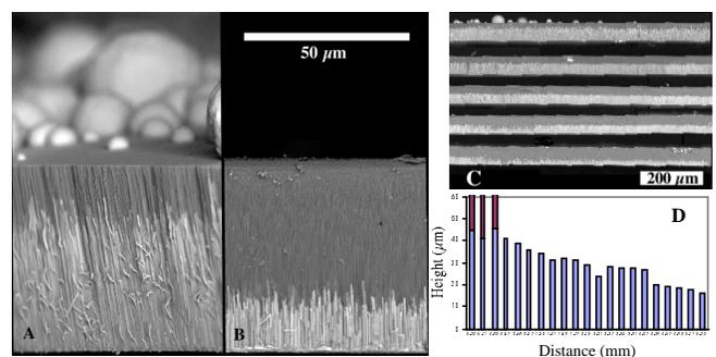
**Figure 2.** (A), (B): SEM images (back-scattered electrons) showing the edge points of a Cu filled membrane, deposited using a lateral gradient of  $-0.8$  V to  $-0.6$  V, respectively. (C), top to bottom: SEM image showing the entire cross-section of the membrane filled with electrodeposited Cu gradient. (D) A graph showing average measured heights of the deposited Cu (the region where Cu is deposited outside the membrane as 'mushrooms' is marked).
