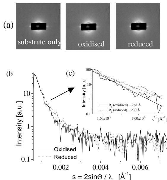
Figure 1 - Scattering from PVF films on glassy carbon substrate. 2D patterns (a) and radially averaged, substrate-reduced (i.e. background subtracted) 1D SAXS profiles (b) highlighting the structural expansion of the polymer chains
