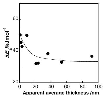
Fig.1. Variation of  $\Delta E_a$  of the electrical conductivity with the apparent average thickness of the liquid phase for  $\alpha$ - $\text{Al}_2\text{O}_3$  powder/ TMPA-TFSI coexisting system.
