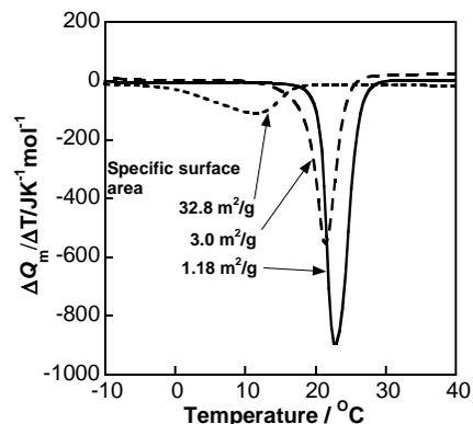
Fig.2. DSC spectra of  $\alpha$ - $\text{Al}_2\text{O}_3$  powder/ TMPA-TFSI coexisting system. Melt content: 30vol%.
