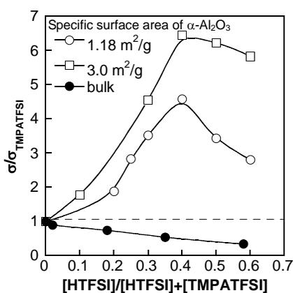
Fig.3. Variation of normalized electrical conductivity at 30°C and the value of  $\Delta E_a$  with  $\text{H}^+$  content for  $\alpha$ - $\text{Al}_2\text{O}_3$  powder/ [TMPA-H]TFSI coexisting system.
