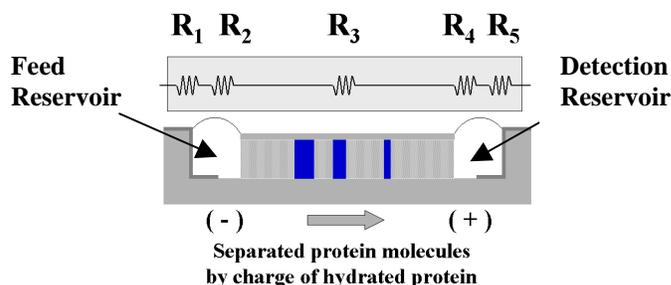
Figure 1 Schematic diagram of electrophoresis in microchannel and its resistance model
