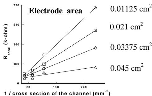
Figure 2  $R_{\text{total}}$  changes with different channel cross-section area and detection electrode size
