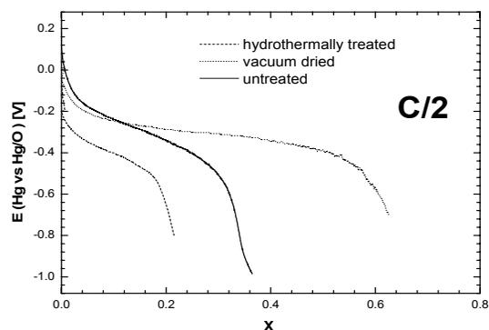
**Figure 1** Potential vs. relative utilization curves for different EMD samples continuously discharged at C/2. Sample assignment is given in Figure inset.
