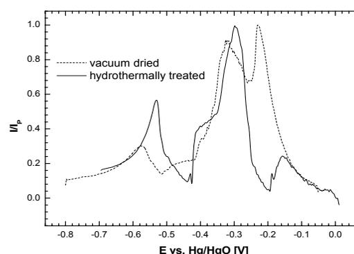
**Figure 2** Linear scan voltammograms of different EMD samples. Polarization rate was 3 μV/s. Sample assignment is given in Figure inset.
