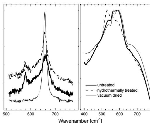
**Figure 3** Raman (left) and infrared spectra (right) of different EMD samples. Sample assignment is given in Figure inset.
