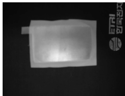
Fig. 1. The Li anode laminated with asymmetrically coated membrane as an anode protection layer and bulk polymer electrolyte(Ni-mesh current collector, coated membrane thickness: 30\mu\text{m} , electrode size: 3\times 5\text{ cm}^2 ).
