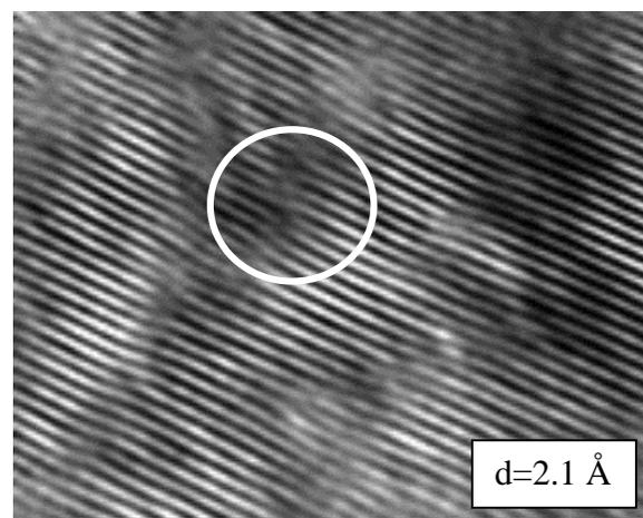
Fig.2 Lattice image of the dislocation in a LNCO grain after cell cycling and power fade.
