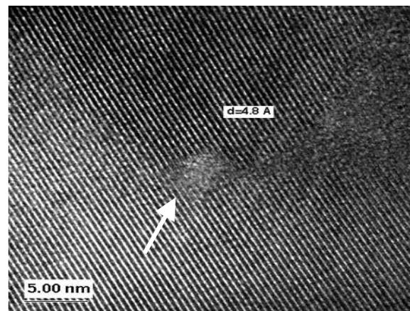
Fig.3 Lattice image of small disordered area (marked by and arrow) & lattice expansion in a LNCO grain.
