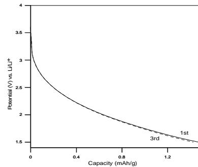
Fig. 3. Discharge profiles of  $\text{Li}_{0.1}\text{La}_{0.9}\text{MnO}_3$  cathode at the current density of  $0.1\text{ mA/cm}^2$
