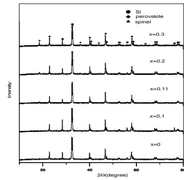
Fig. 1. XRD patterns of powdered  $\text{Li}_x\text{La}_{1-x}\text{MnO}_3$  powder after calcination at  $900^\circ\text{C}$  for 24 hr.
