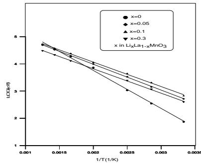
Fig. 2. Conductivity of  $\text{Li}_x\text{La}_{1-x}\text{MnO}_3$  plotted as a function of  $1/T$
