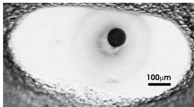
Figure 2. A pit (black round spot) can be observed during the experiment, the darker area at the edge is covered with insulating mask.
