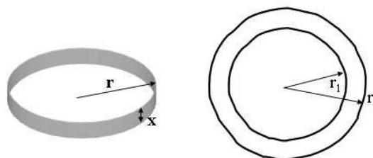
Figure 3. The active pit area is the side area of the cylindrical disc,  $2\pi rx$ . The pit radius increase with time, and therefore the active surface is changing instantaneously.
