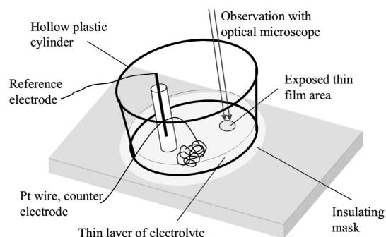
Figure 1. The schematic diagram for 2-D pit growth setup.
