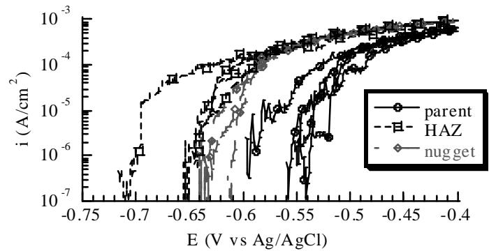
**Figure 2** Anodic polarization curves for FSW B in 0.1 M NaCl across the weld using micro-electrochemical device.
