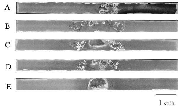
**Figure 1** Immersion test on FSW 2024-T351 with different welding parameters after 24 hr exposure in 0.1 M NaCl.
