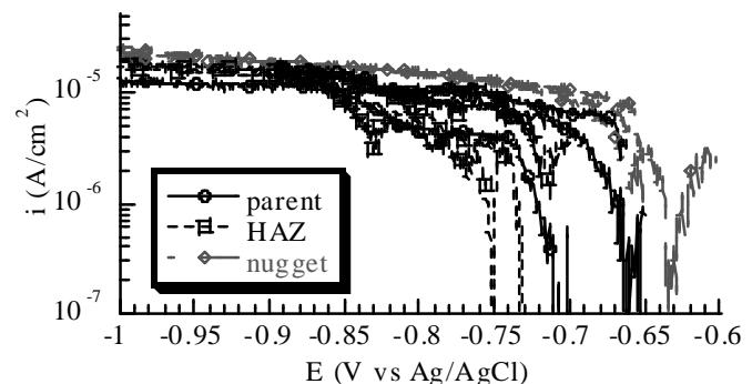
**Figure 3** Cathodic polarization curves for FSW B in 0.1 M NaCl across the weld using micro-electrochemical device.
