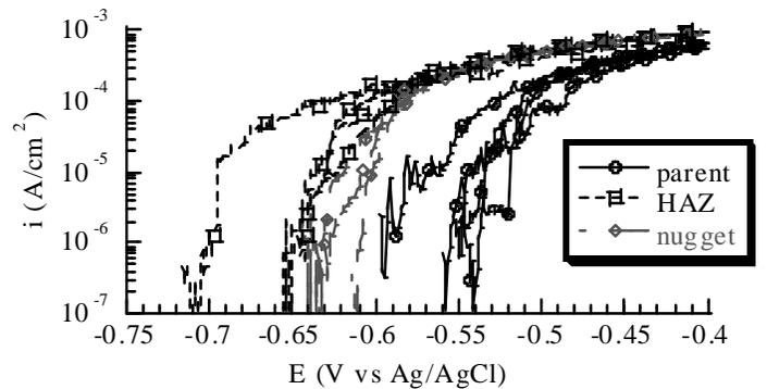
**Figure 2** Anodic polarization curves for FSW B in 0.1 M NaCl across the weld using micro-electrochemical device.
