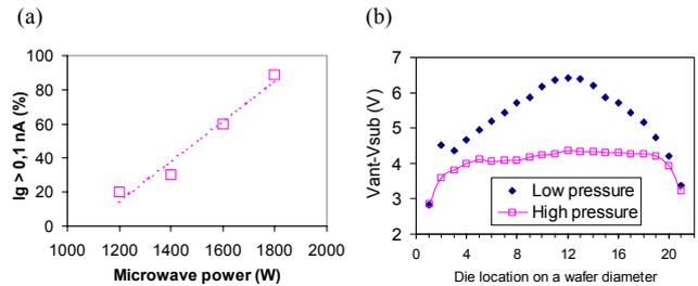
Fig. 2 (a) Charging degradation vs. microwave power in a ECR-CVD tool. (b) Positive antenna voltage vs. the process pressure in a PECVD tool.
