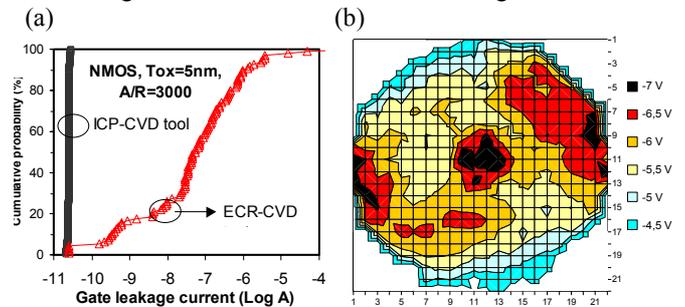
Fig. 1 (a)-Metal antenna structure degradation vs. the CVD tool. (b)- Negative antenna voltage in ECR-CVD tool.
