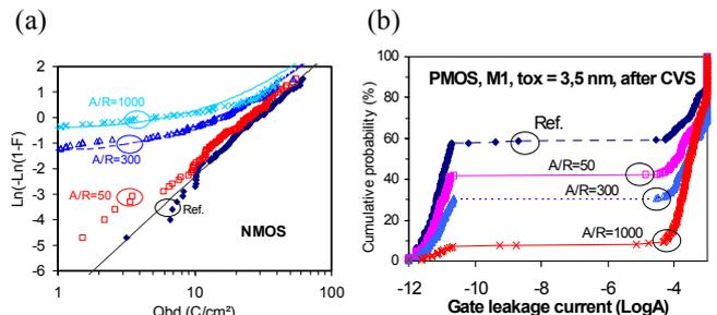
Fig.3 CVD charging impact on Qbd results (a) and gate leakage after a voltage stress (b). Tox =3.5nm.
