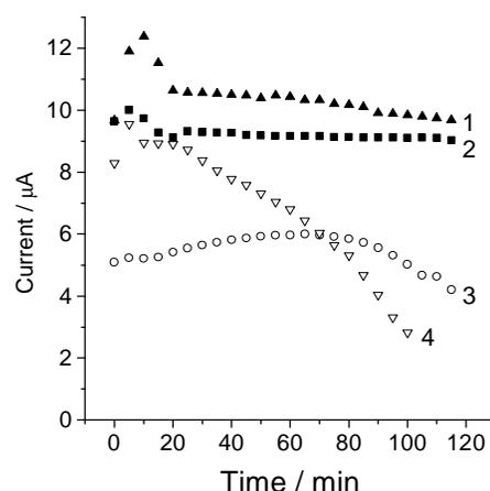
Figure 1 Variation in anodic peak current of CVs for 100  $\mu$  M of p-nonylphenol (1,4) and p-hexylphenol (2,3) obtained at ECR carbon (1,2) and GC (3,4) electrodes.
