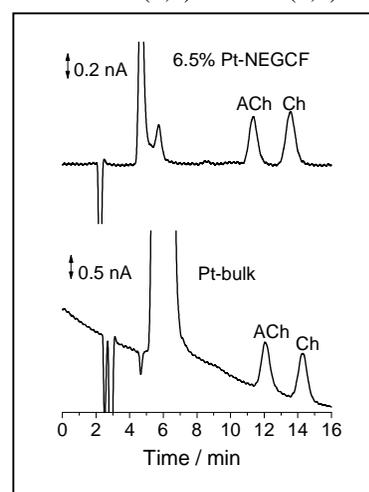
Figure 2 Chromatograms of ACh and Ch (100 fmoles) at carbon and Pt bulk electrodes containing dispersed Pt nano-particles .
