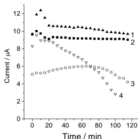
Figure 1 Variation in anodic peak current of CVs for 100 μM of p-nonylphenol (1,4) and p-hexylphenol (2,3) obtained at ECR carbon (1,2) and GC (3,4) electrodes.
