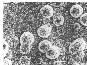
Figure2: SEM Micrographs (1500x) of Zn-Ni alloy coated surface.
