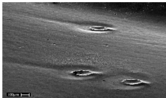
Figure 4. SEM image of H<sub>2</sub> bubble traces on a stationary nickel deposit prepared at -1 V/SCE from a Watts bath containing 5 mM 2-butyne-1,4-diol - B = 0.6 T.
