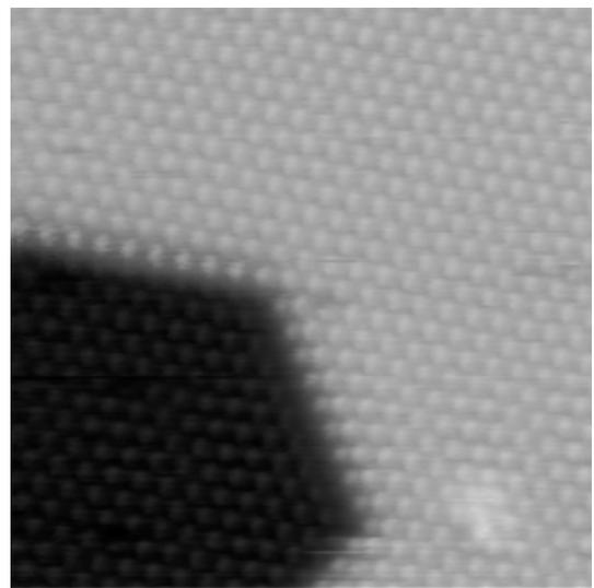
Fig. 2: Commensurate  $(\sqrt{7} \times \sqrt{7})R19.1^\circ S^{2-}$ -adlayer on Cu(111)
