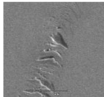
Fig. 3. Typical post-CMP  $\mu$ -scratch.
