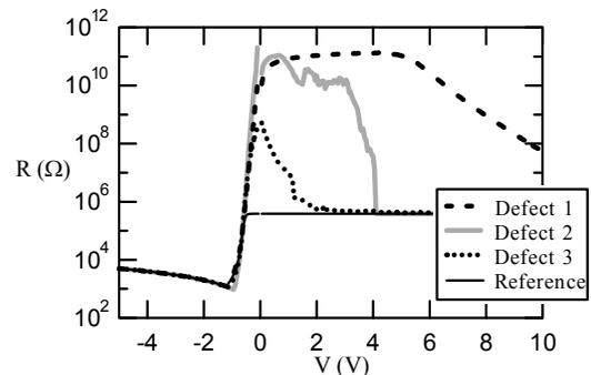
Figure 2. Resistances of the defects as measured by Nano-prober.
