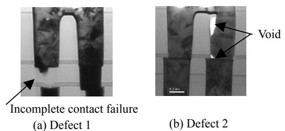
Figure 3. Cross-sectional TEM images of the detected defects after the measurement of I-V characteristics.
