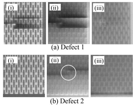
Figure 1. Examples of the SEM images of the defects at irradiation energies of (i)1.0, (ii)2.0, and (iii)3.0 keV.
