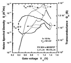
Figure 1: Linear Kink Effect related noise contribution to the drain current noise power spectral density in a FD (at  $V_{BG}{=}0$  V and –20 V) SOI n-MOSFET with L=1  $\mu m$  and W=10  $\mu m.$
