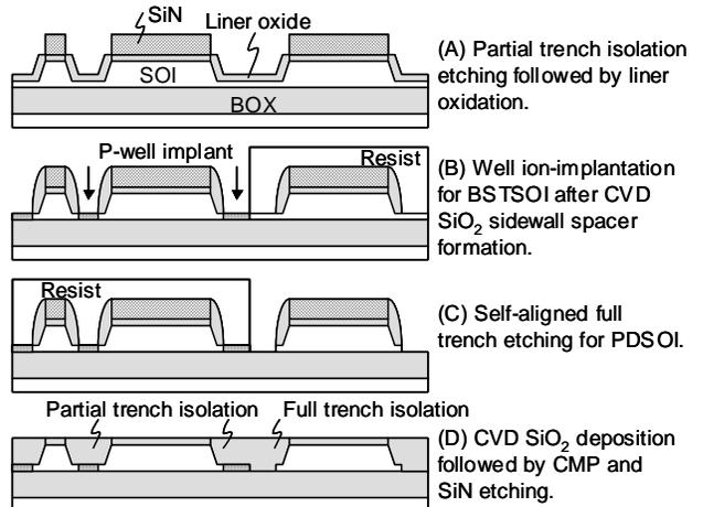
Fig.3 Process sequence of self-aligned dual trench isolation
