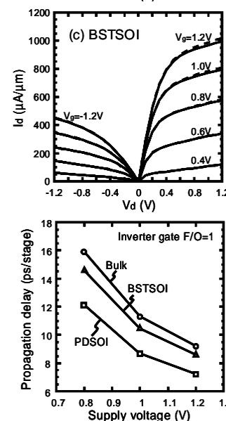
Fig.5 Propagation delay of inverter gate. Lg=60nm, Wn=0.9μm, Wp=1.44μm.
