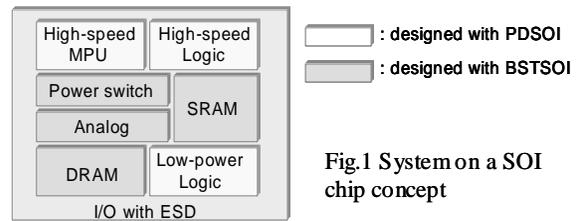
Fig.1 System on a SOI chip concept
