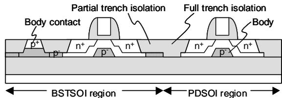
Fig.2 PDSOI and BSTSOI structures
