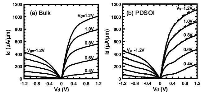
Fig.4 Output characteristics of (a) Bulk, (b) PDSOI, and (c) BSTSOI CMOS with Lg=60nm. Solid line shows raw DC measurement data with SHE. Broken line shows SHE eliminated data.
