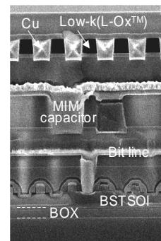
Fig.6 SEM view of embedded DRAM on BSTSOI.
