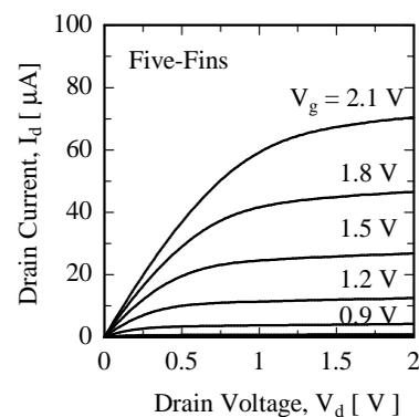
Fig. 4. I<sub>d</sub>-V<sub>d</sub> characteristics of the fabricated FXMOSFET with five-Fins.
