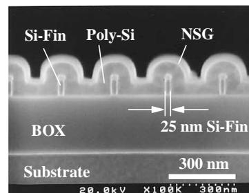
Fig. 2. Cross-sectional SEM image of the fabricated MFXMOSFET with 5-Fins.
