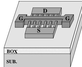
Fig. 1. 3-D schematic diagram of the proposed multi-Fin XMOSFET structure.
