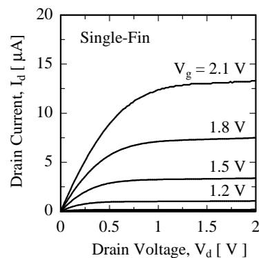
Fig. 3. I<sub>d</sub>-V<sub>d</sub> characteristics of the fabricated FXMOSFET with single-Fin.
