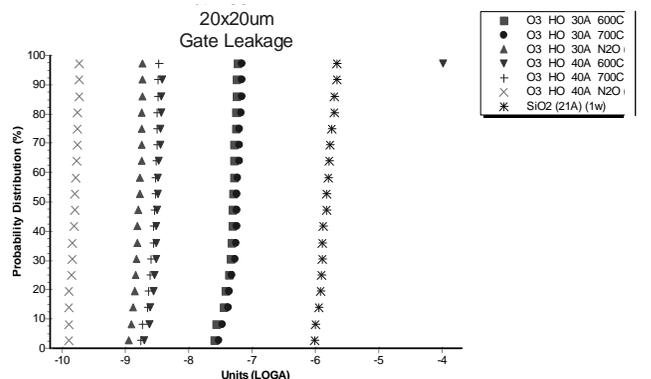
**Figure 2** Probability distribution of gate leakage in NMOS devices fabricated from 30 and 40 Å thick ALD HfO<sub>2</sub> layers with O<sub>3</sub> – based pre-treatment.
