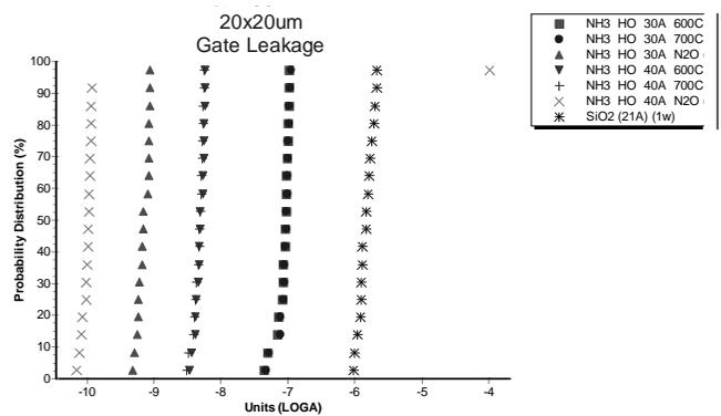
**Figure 1** Probability distribution of gate leakage in NMOS devices fabricated from 30 and 40 Å thick ALD HfO<sub>2</sub> layers with NH<sub>3</sub> – based pre-treatment.
