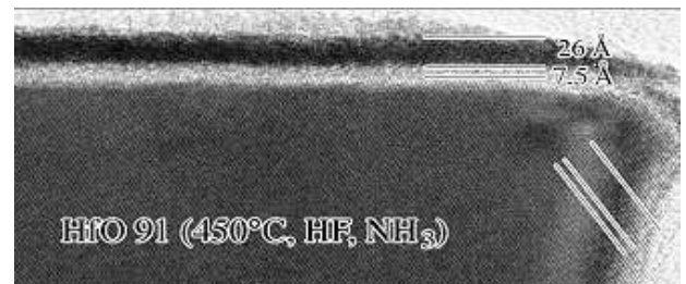
Figure 1. HRTEM image of a 2.6 nm HfO 2 layer formed by liquid injection MOCVD at 450°C following a HF / NH 3 670°C surface preparation. The interface oxide layer is 0.75 nm.
