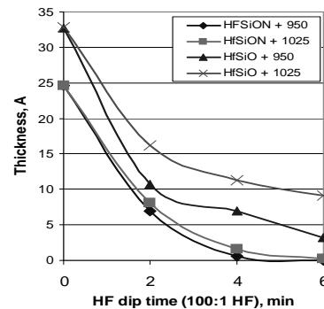
Fig. 2, Etching of HfSiO and HfSiON in dilute HF.
