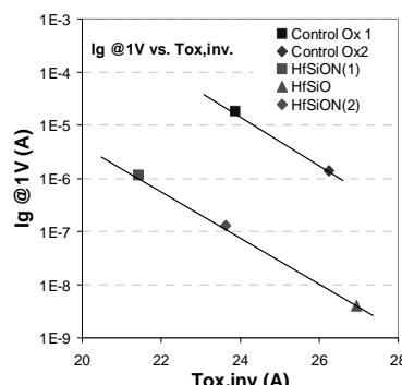
Fig. 3, Gate leakage current as a function of Tox,inv.
