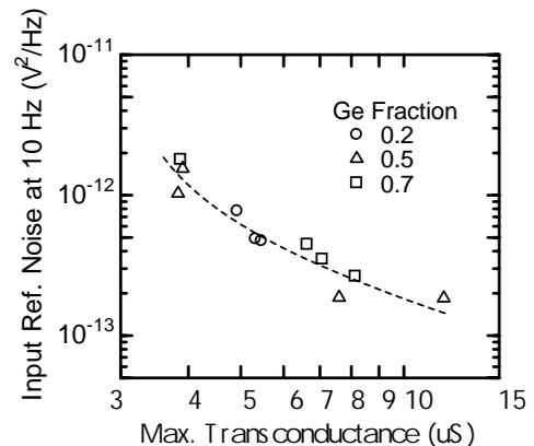
Fig. 3 Relationship between the noise power and the maximum linear transconductance.
