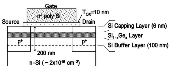
Fig.1 Schematic cross section of SiGe-channel pMOSFETs
