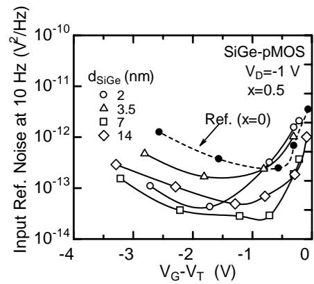
Fig.2 Noise power at 10 Hz as a function of  $V_G - V_T$ . Ge fraction  $x=0.5$ .
