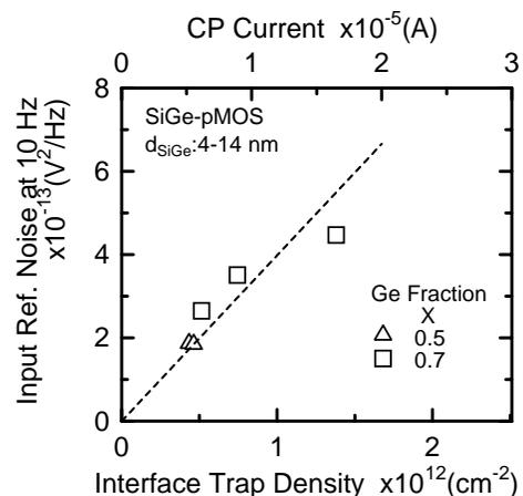
Fig. 4 Correlation between the measured hetero-interface trap density and the low frequency noise level in the current flowing in the SiGe-channel
