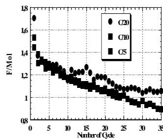
Fig 3 : Evolution of the faradaic yield as a function of the number of cycles for different discharge-charge rates.
