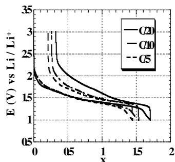
Fig.2 : Chronopotentiometric behaviour of  $\text{Li}_2\text{Ti}_3\text{O}_7$  in 1M  $\text{LiClO}_4/\text{PC}$ .
