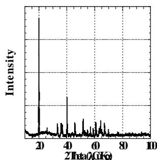
Fig.1 : Powder X-ray diffraction pattern of  $\text{Li}_2\text{Ti}_3\text{O}_7$  obtained at 1050°C/24H after quenching.
