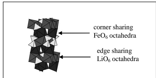
Figure 1. Structure of LiFePO<sub>4</sub> showing connectivity of framework components.
