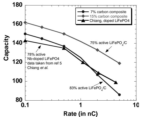
Figure 1. Comparison of electrochemical performance as a function of rate for our LiFePO<sub>4</sub>/C materials (75% active and 83% active; C/2 rate ~ 85mA/g); and data reported for Li<sub>0.99</sub>Nb<sub>0.01</sub>FePO<sub>4</sub>, taken from reference 3 (78% active; C/2 rate ~ 75 mA/g)
